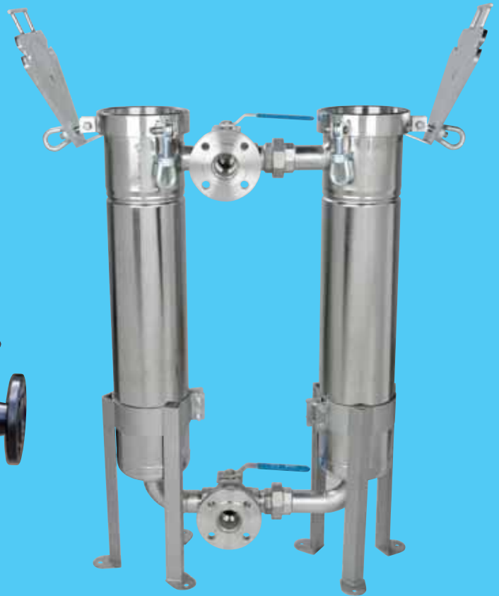
Two RBFH housings manifolded together and fitted with valves to enable use in a continuous process. One filter bag can be changed out whilst the other housing is in use.
